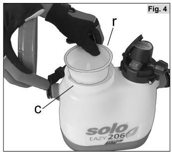
The basket in the filling neck ( $\mathbf{c}$ ) of the liquid tank contains a filter screen( $\mathbf{r}$ ).
